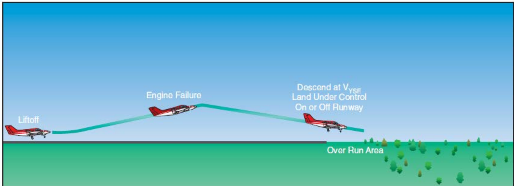
Figure 12-12. Engine failure on takeoff, inadequate climb performance.
