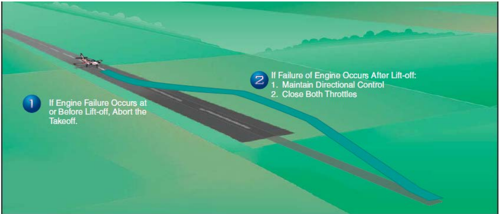
Figure 12-11. Engine failure on takeoff, landing gear down.
