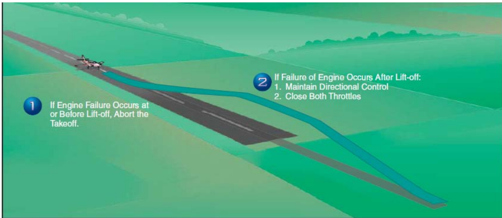
Figure 12-11. Engine failure on takeoff, landing gear down.
