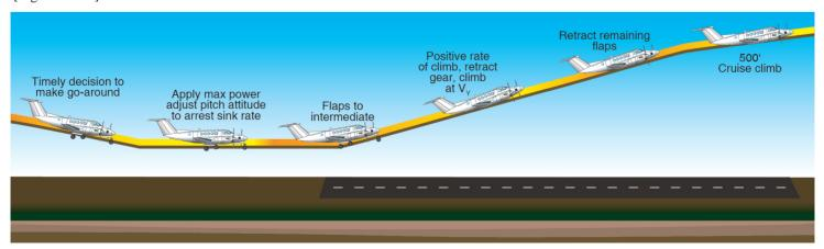
Figure 13-11. Go-around procedure.
