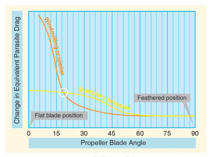
Figure 13-3. Propeller drag contribution.
