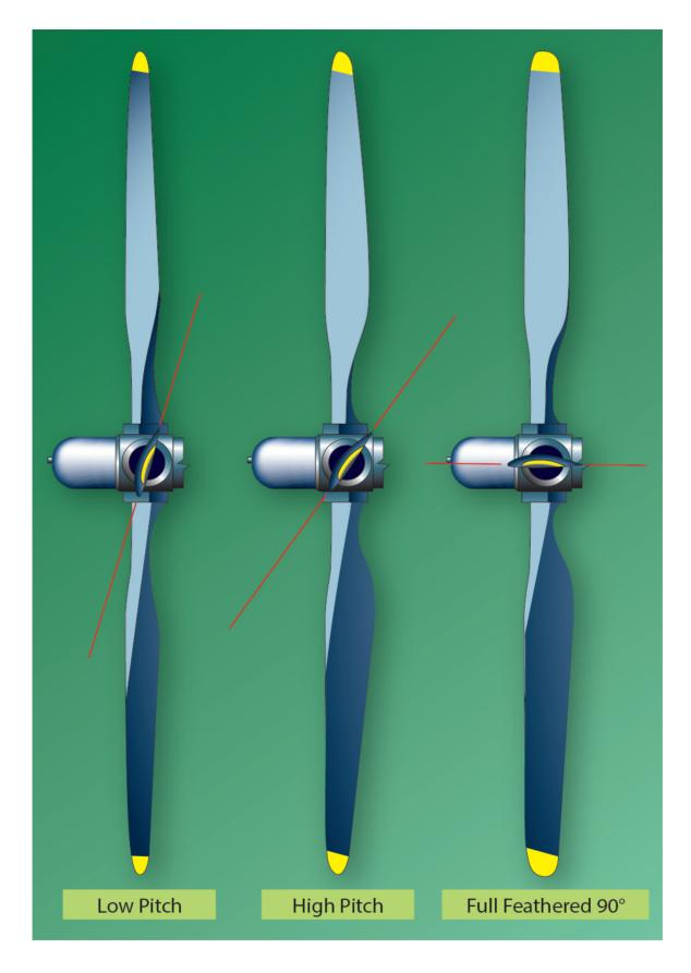
Figure 13-2. Feathered propeller.
